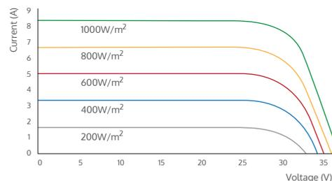
\* Irradiance of 1000W/m<sup>2</sup>, spectrum AM of 1.5 and cell temperature of 25°C
